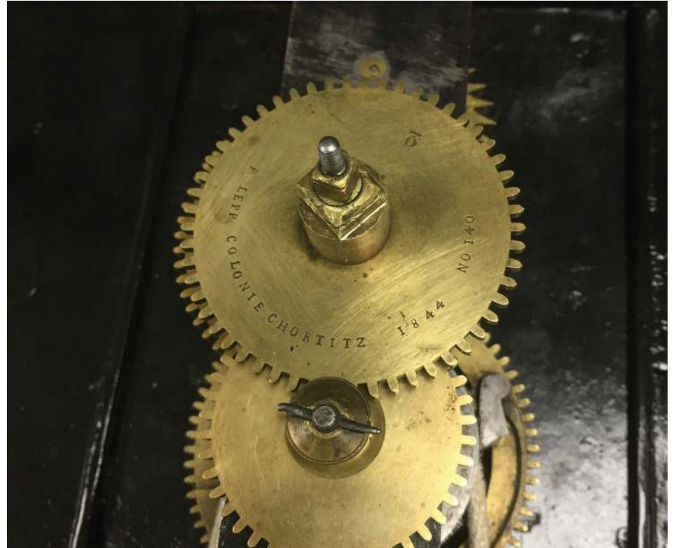
The Lepp clock's movement. We know this is a Lepp clock because Peter Lepp stamped his mark into the hour wheel.
